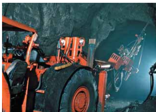
Fig. 10. A photograph of the OKU-jumbo, developed in the 1960's
