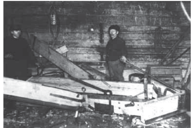
Fig. 19. Making a road grader at the Möhkö blacksmiths' workshop in the 1930's. Photograph courtesy Ilomantsi Museum Foundation
