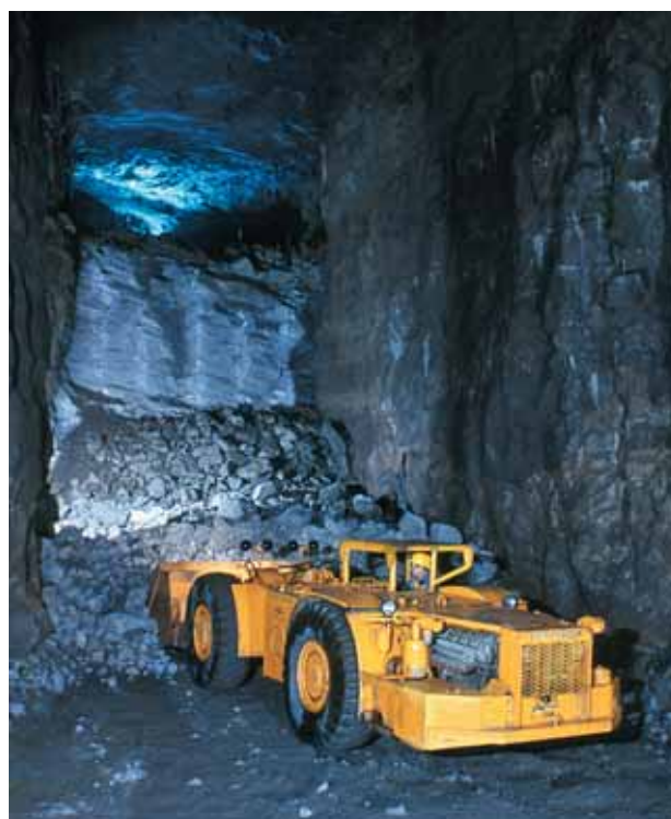
Fig. 11. Wagner front-end loader hauling ore. The capacity of the bucket was 35 cubic meters
